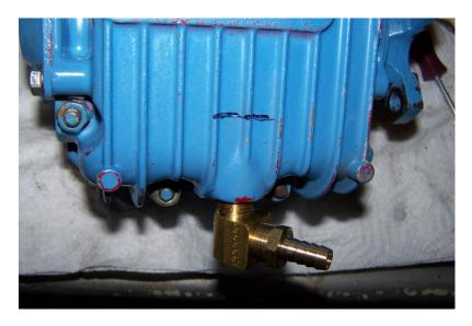
The scribed line on the case is the Fluid level when full.. you will be able to reference the Level in the hose if you use transparent hose on your installation. You'll be able to check the Oil level at a glance this way.
