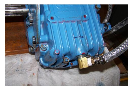
When using Vinyl hose like this **you must use Synthetic ATF**. Normal ATF will dissolve the hose. For long life I'd use synthetic ATF always. Resists heat and reduced wear.
