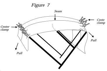
Start at the centered clamps and stretch the cloth out between the forward and aft bows. Clamp along the bows on three to six-inch intervals drawing the fabric tightly as you go.
