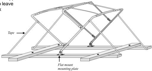
Frame is ready for fitting - strapping tape holds the bows in place
