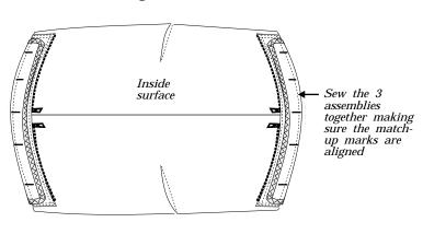
Lay the fore and aft sleeves and tails in position on the cover piece
