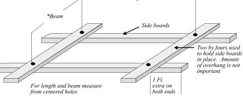
\*(Desired width of bimini mount from leg to leg)
