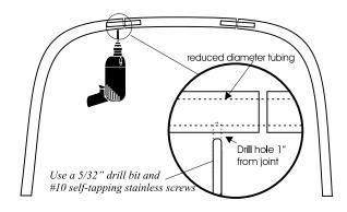
With each bow lying on a flat surface, use a 5/32nds inch drill bit to make two pilot holes (one on each side of the joint where the two frame pieces meet). Drill through both the frame piece and the reduced tubing. Be sure to drill up from the bottom of the frame so that, when the screw is inserted, it will not come in contact with the fabric. If a center punch is used first to make a "dimple" for starting the hole, drilling will be easier .
