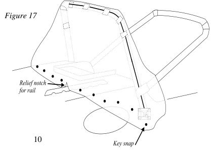
rails and any other protrusions on the cabin top (Figure 17). The last snap should be located on a line extended from the longest bow leg (Figure 18). Any snap mounted aft of this location would have to be undone in order to fold the frame forward.
