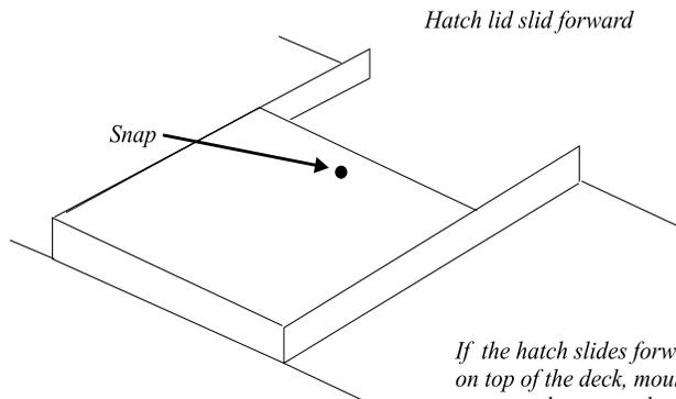
*If the hatch slides forward on top of the deck, mount the snaps to the outer edge of the hatch.*
